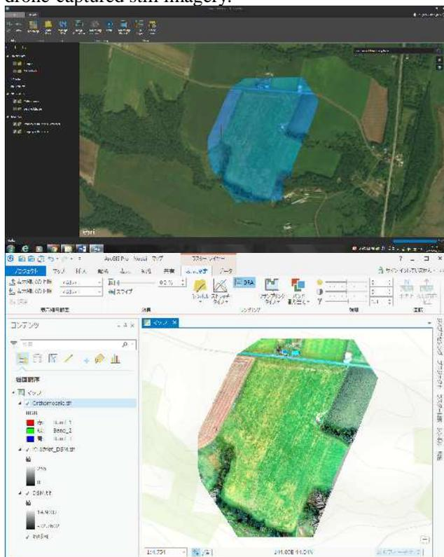
Fig. 7 Orthomosaics from drone-captured imagery
